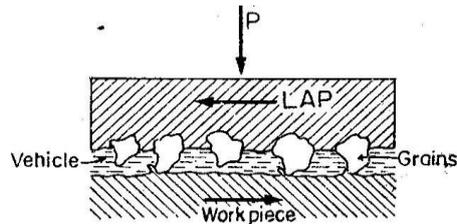
Fig.1 Scheme of lapping process
