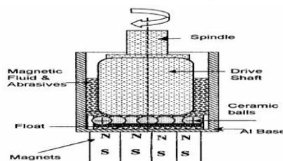
Fig.6 Magnetic Float polishing.
