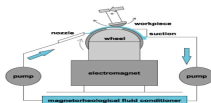
Fig 8. Magnetorheological Finishing Machine
