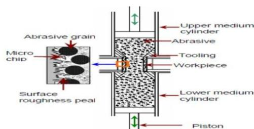
Fig.5 Abrasive flow machining
